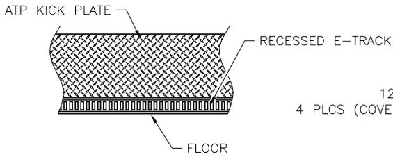
E-TRACK LOCATED AT THE BOTTOM OF THE WALL AND RUN THE FULL LENGTH OF SIDE WALLS AND V-NOSE WALL OPPOSITE FRONT RAMP DOOR
