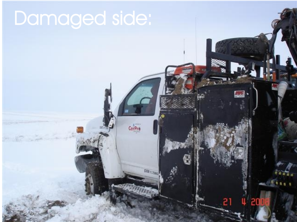
Scrape, small crack to fender:
