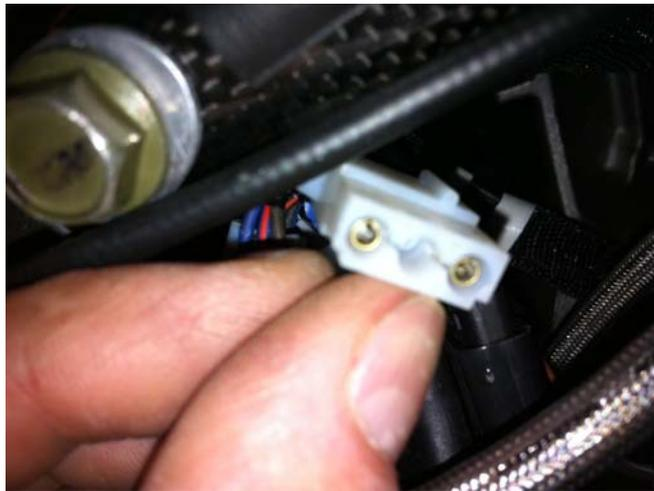
The White and Yellow Teth-Air wires are connected to this white plug. polarity does not matter as this plug supplies AC voltage.
