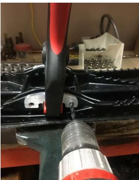
Step 3: With the brace top parallel with the curvature of the top of the ski, drill the 2 holes all the way through with a 17/64" drill.
