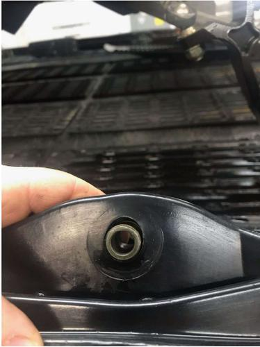
Designed to strengthen the Polaris Gripper Ski mount and reduce wear.
