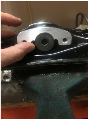
Step 1: Remove the ski and position the brace over the exterior of the ski mounting hole. Match the angle of the cutouts with the webbing internal to the ski as there is a front and rear of the brace.
