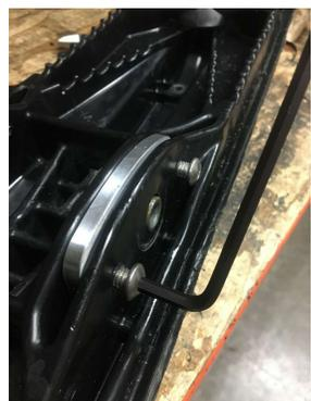
Step 6: Insert the provided bolts and tighten. Note these bolts only need to be snug. The compression of the plastic will lock them from backing out. Step 7: Do the same for the other side of ski and then re-install the ski.
