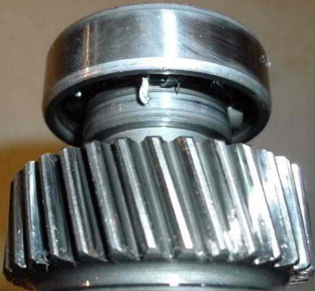
Portions of the cage remained in the bearing, surrounding three of the balls. The loose piece of cage was also in the bearing, held in by the seal. The outer seal was in place, until I popped it off with a screwdriver. Then the loose piece of cage fell out.
