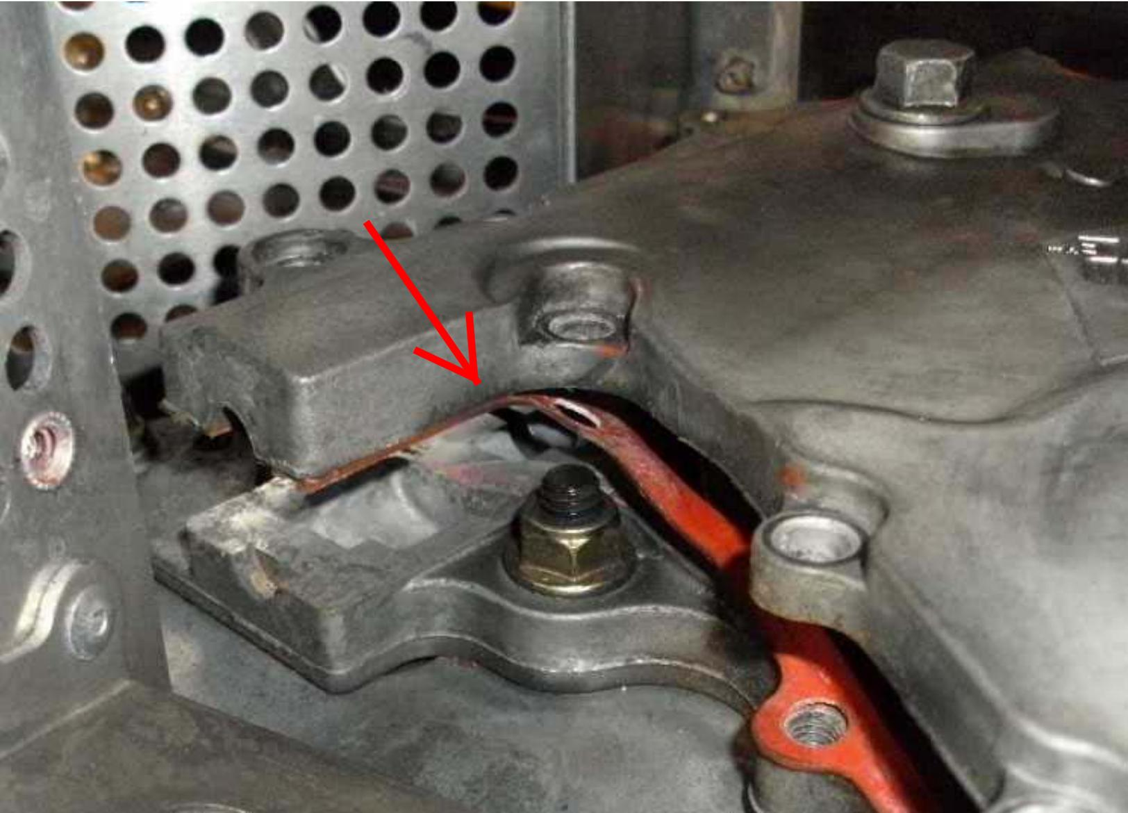
This is what it looks like with the cover removed. The transfer shaft will wiggle free by hand and pull straight up and out - fairly easy. The bad bearing is on the other end of the transfer shaft.
