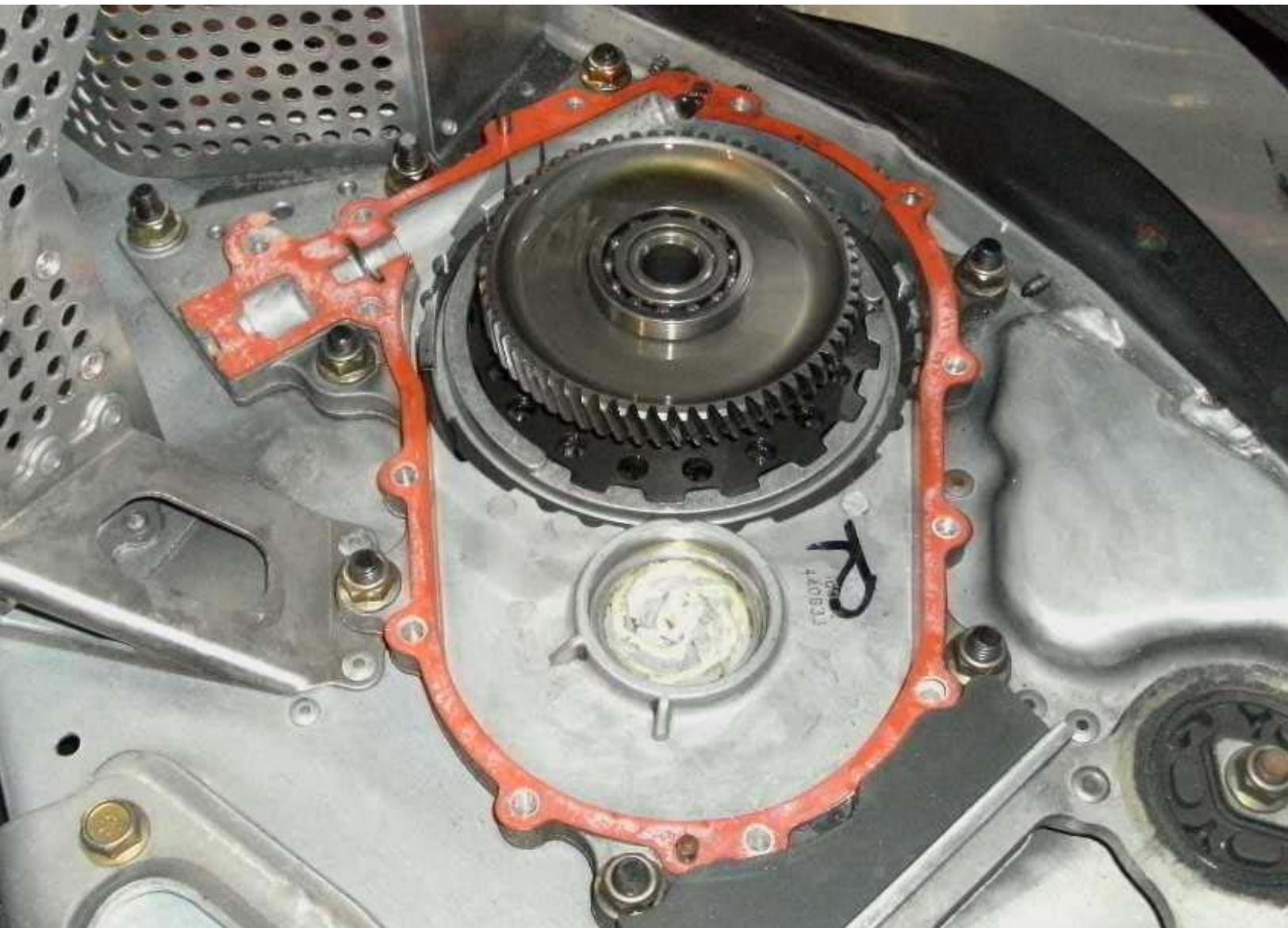
Shrapnel in the DD case!! Removed 2nd snap ring and fished crap out with a magnet. Also through the holes in the drive shaft basket. The DD oil is new and clean. Plan to run it one ride and then flush with fresh oil.
