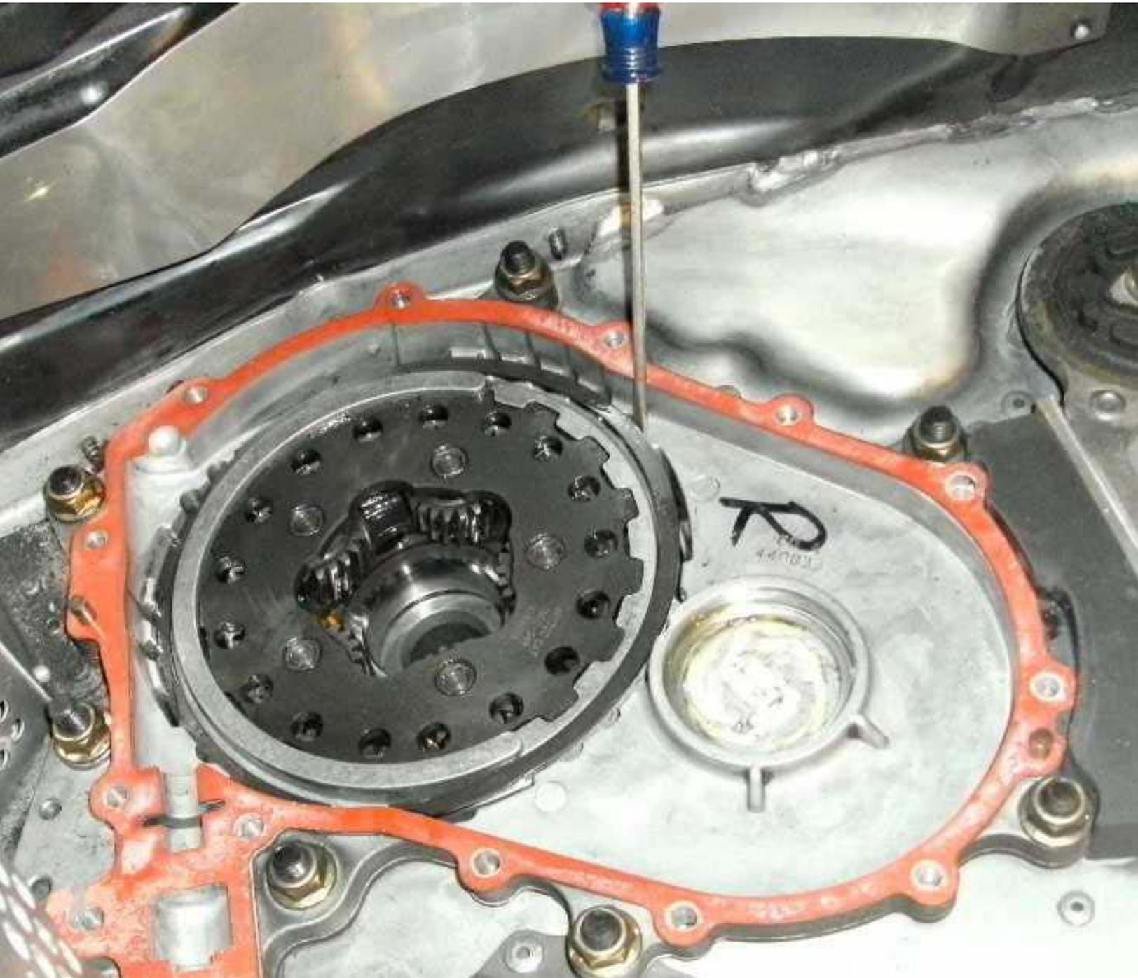
A magnet easily grabbed loose metal parts and debris from the bearing cage. Wiped out every thing with clean paper towels - sludge and small metal flakes.
