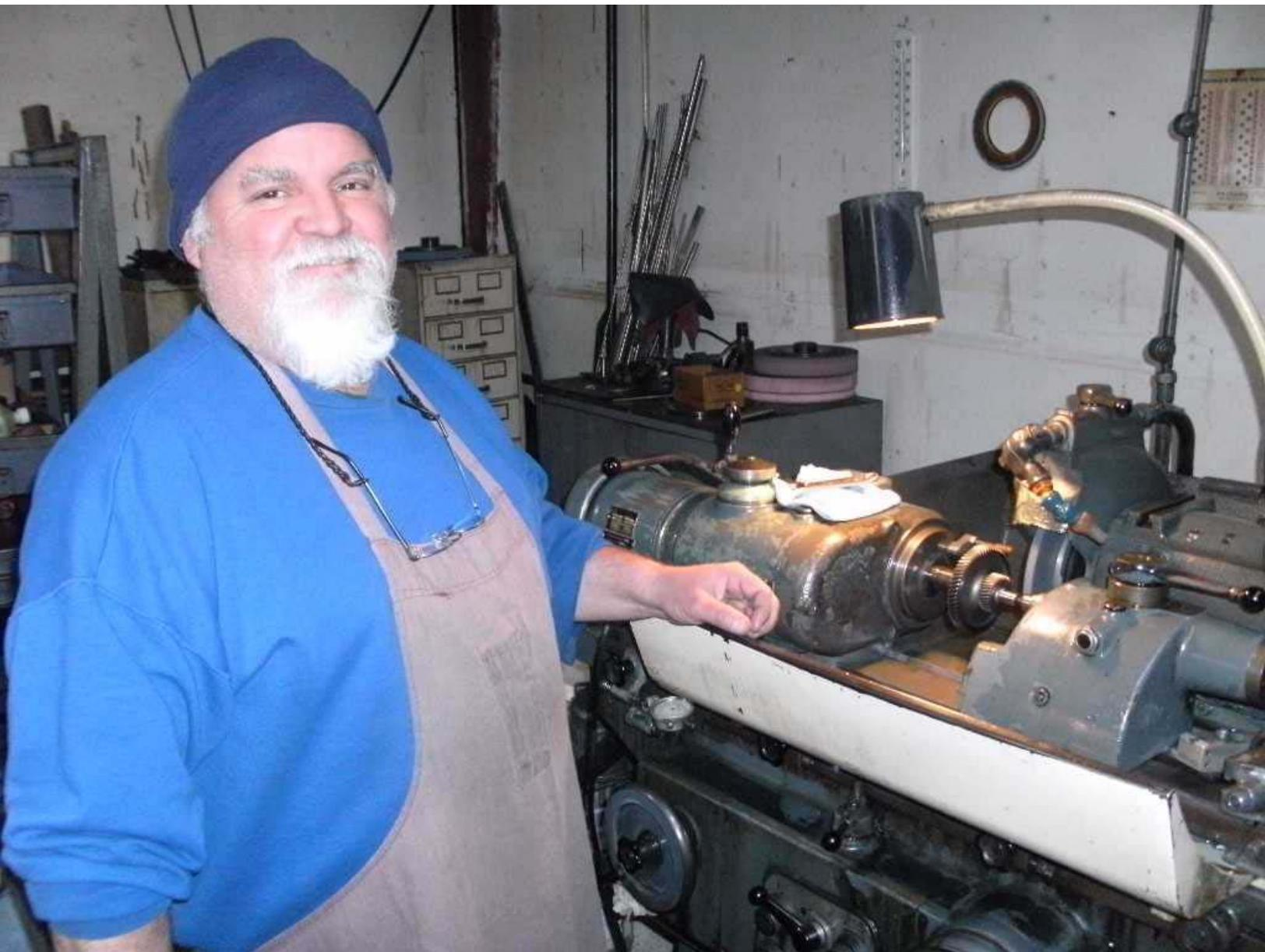
His grinding machine (one of many) is dual centered and liquid cooled. He dresses the stone to cut only on the corner. Doug matched the shaft size, without touching the original shaft surface and moved the shoulder back exactly 0.040". He's a precision guy.
