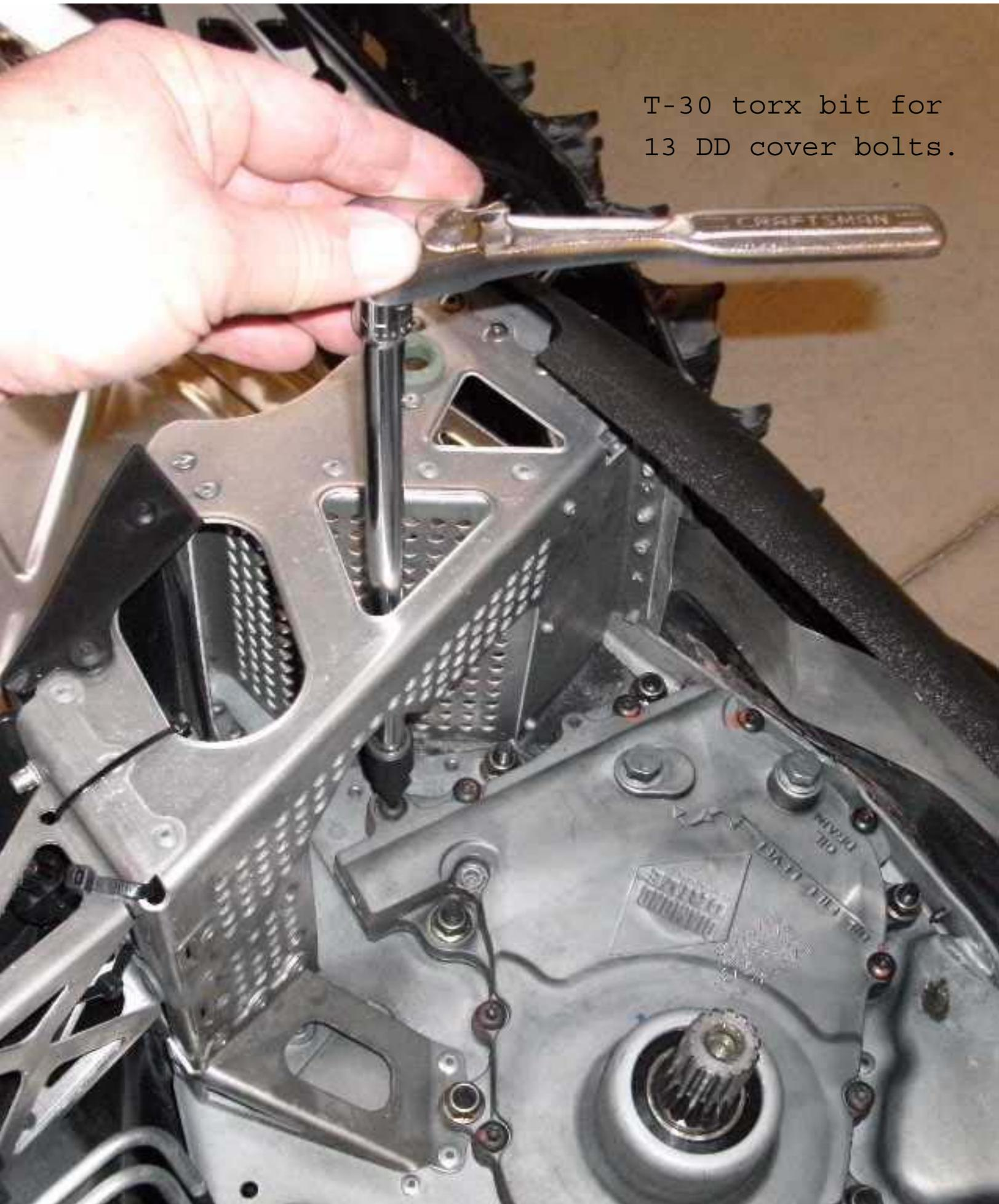
One cover bolt is impossible to get at with a ratchet. Had to use the T-30 bit with a 5/16" wrench. The rest were easy.
