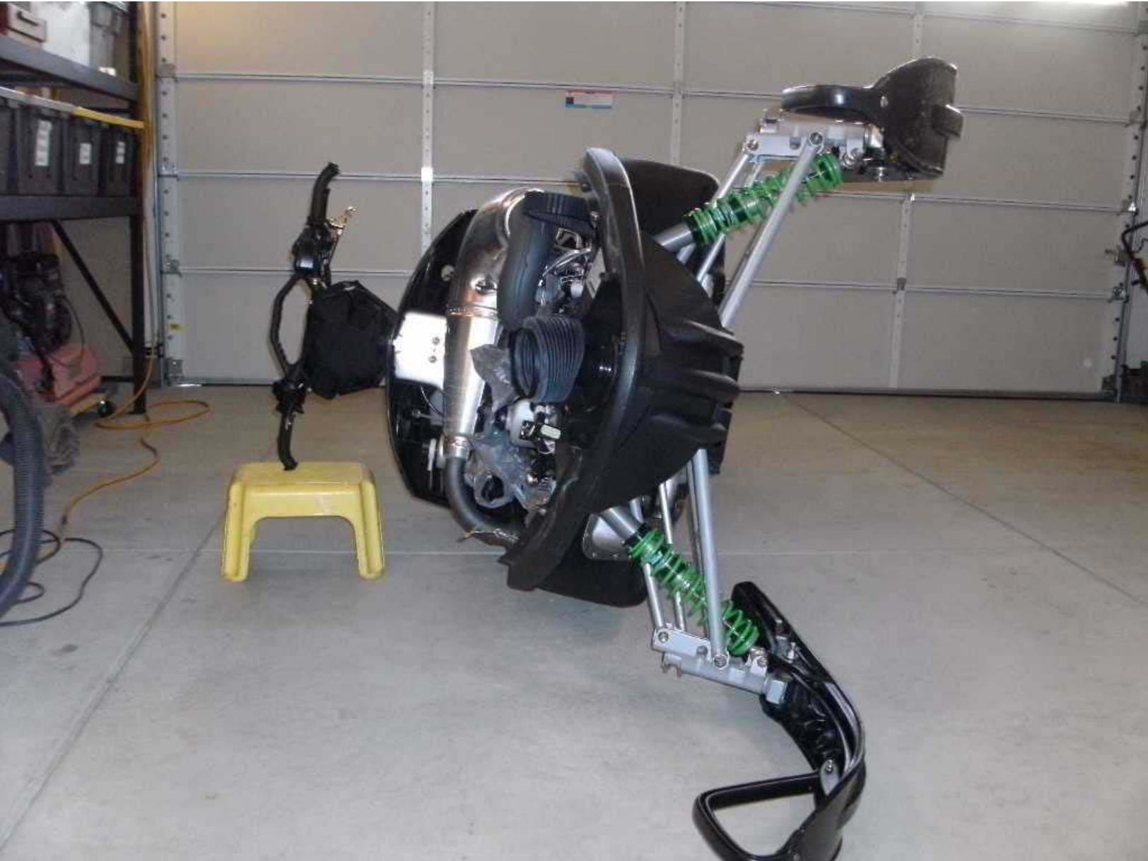
Removed foot pocket brace. Four T-20 torx screws.
