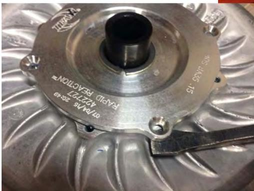
Spin the back sheave to loosen the helix and generally pry off.
