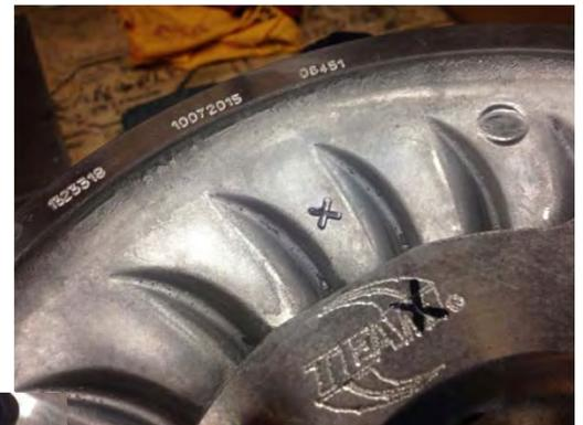
Heat the back sheave with a torch to loosen the thread locker and then remove the 4 bolts with a good quality T27 Torx bit .
