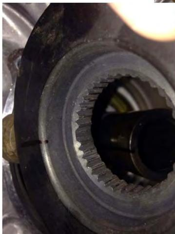
Note the double wide teeth must line up while re-tensioning the spring.
