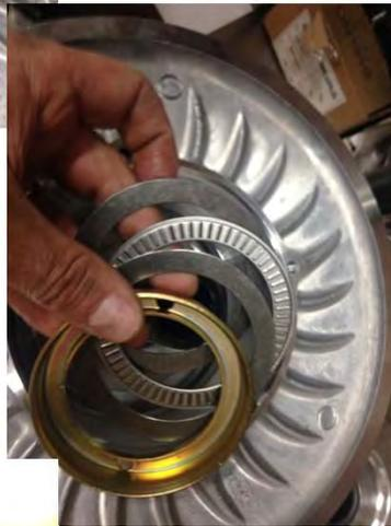
Re-assemble clutch and torque the **helix bolts to 60-80 in-lbs**. Blue Loctite is also recommended by the manufacturer . Torque the **jackshaft bolt to 17 ft-lbs** and also use Blue Loctite.
