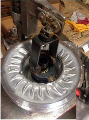
A good clutch press is now required to remove the retainer clip.
