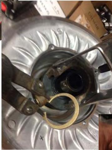
Apply a thin layer of low temperature grease to the roller bearing. Wipe off excess as you only need a thin film .
