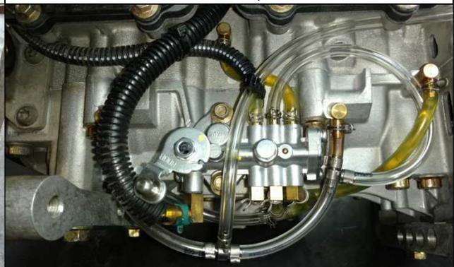
11B) ENSURE THE OIL LINES ARE CORRECT EVEN THE ONES YOU HAVE NOT CHANGED. USE THE ORIGINAL PINCH CLAMPS TO SECURE THE LINES AND MAKE SURE THE LINES ARE PROPERLY TIED TO PREVENT RUBBING ON THE ENGINE OR CHASSIS.
