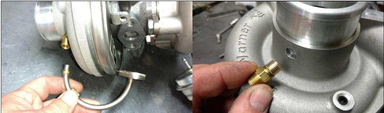
1) REMOVE MUFFLER AND TURBOCHARGER FROM SLED. REMOVE THE OIL LINE LOOP TUBE FROM THE TURBO CENTER SECTION/COMPRESSOR HOUSING.
