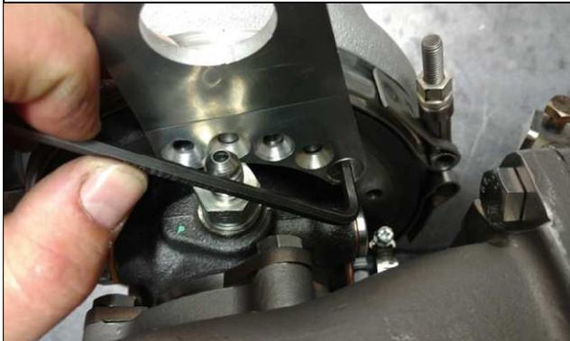
5) USING A 4MM ALLEN L-WRENCH REMOVE THE 3 SCREWS HOLDING THE WASTEGATE BRACKET AND REMOVE IT.
