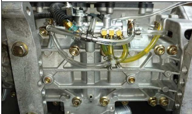
11A) USING PICTURES 11A AND 11B FOR A REFERENCE INSTALL THE NEW OIL LINE ASSEMBLY AS SHOWN AND SECURE PROPERLY.
