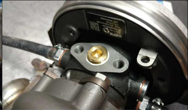
10) TURN THE TURBOCHARGER OVER AND FILL THE CENTER SECTION FROM THE BOTTOM DRAIN HOLE WITH CLEAN TWO STROKE OIL LEAVING A 1/2" AIR SPACE FROM THE TOP. APPLY THREAD SEALANT AND INSTALL THE 3/8" BRASS PLUG.
