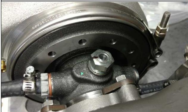
7) UNTHREAD THE FITTING AND USING A THREAD LOCKING COMPOUND PRESS THE OIL CHECK VALVE IN ALIGNED WITH THE MARK YOU MADE. REINSTALL THE FITTING AND TIGHTEN.
