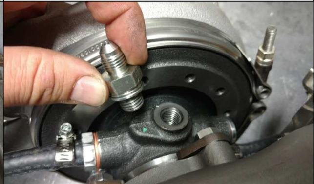
6) REMOVE AND REPLACE THE OIL LINE INLET FITTING WITH THE NEW FITTING. TIGHTEN AND MARK THE FITTING WHERE THE OIL LINE SHOULD POINT WITH THE WASHER AND O-RING INSTALLED. IT SHOULD POINT TO THE REAR OF THE SLED WHEN THE TURBOCHARGER IS INSTALLED.
