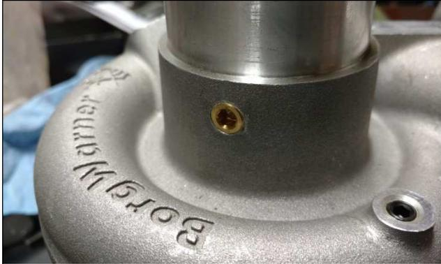
3) PLUG THE HOLE IN THE COMPRESSOR HOUSING WITH THE 1/8" BRASS PIPE PLUG. USE THREAD SEALANT AND TIGHTEN.
