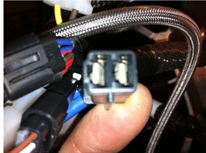
The Green and Brown Teth-Air wires Plug into this black plug. The gray wire is Not used and can be taped off or cut off.
