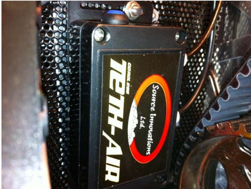
We decided that the best location was ahead of the exhaust side foot rest. The picture shown is with a Skinz mesh in place which make it easy to mount. The LED indicator and push-button is easy to access with the side panel open. There is about 2 cm clearance to the belt drive. Use nuts and bolts with lock washers or Loctite so the Teth-Air can't vibrate loose. Wire-tie any loose wires to keep them out of the drive belt.
